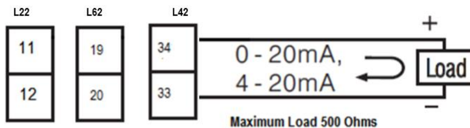
2-24 Retransmission Wiring - Current
