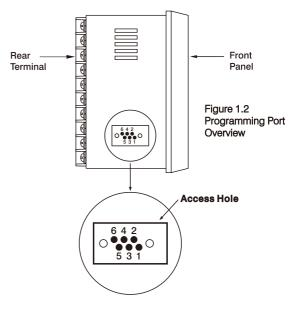
A special connector can be used to touch the programming port which is connected to a PC for automatic configuration, also can be connected to an ATE system for automatic calibration and testing.
