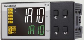
The IA10 Indicator and Alarm Unit offers two input channels capable of performing arithmetic operations  $(+, -, \times, \div)$  for enhanced data processing. Its three-color LCD displays provide clear and intuitive readability, with the main and secondary screens supporting five-digit values and up to four decimal places. A dedicated status and unit display section ( $^{\circ}\text{C}$ ,  $^{\circ}\text{F}$ , PU) on the left ensures quick reference.
