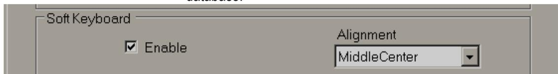
**Soft keyboard:** If enabled, it is possible to control the keypad appearance during run time. For example, if “alignment” is selected as the Middle centre, then, when the keypad appears during run time, it will be located in the middle-centre of the screen
