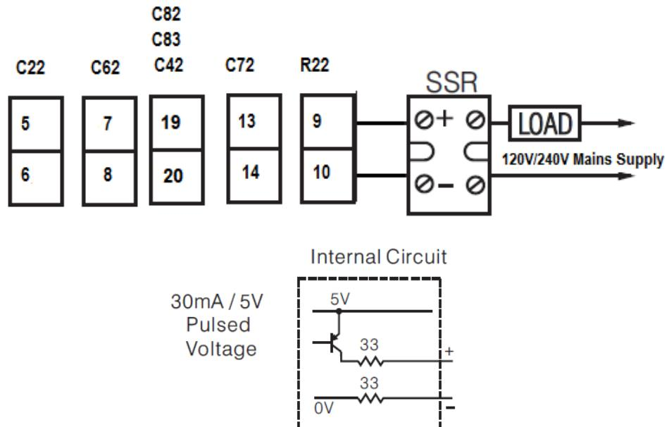
**2-33 Output 2 Pulsed Voltage to Drive SSR**
