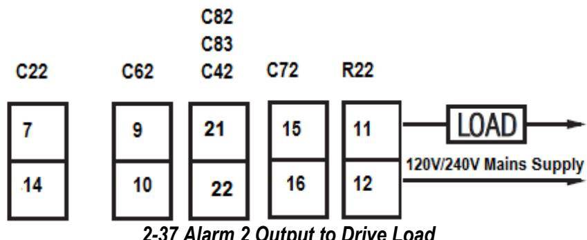
**2-37 Alarm 2 Output to Drive Load**
