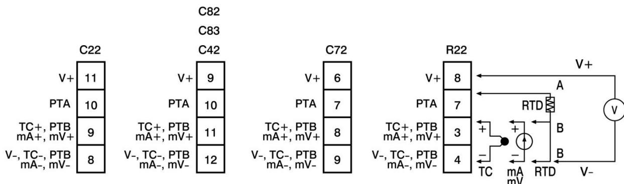
2-25 Sensor Input Wiring
