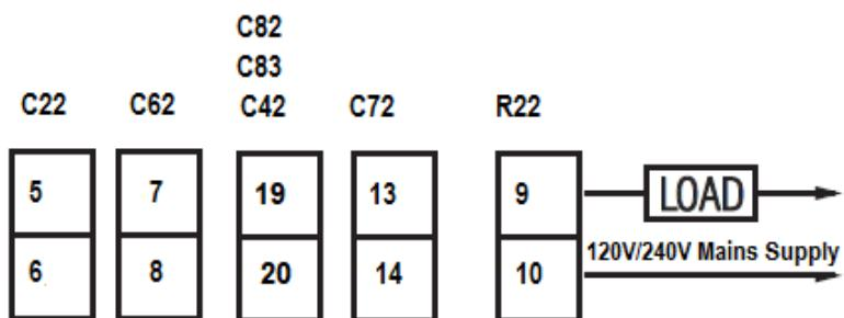
**2-36 Alarm 1 Output to Drive Load**
