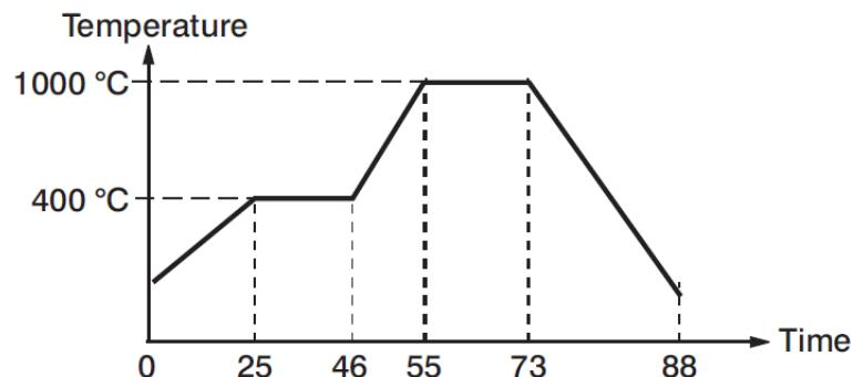
**4-12 Temperature Profile of the Heat Treatment Chamber**
