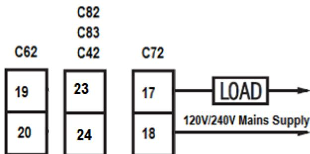
**2-38 Alarm 3 Output to Drive Load**
