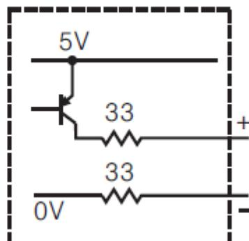
**2-28 Output1 Pulsed voltage to Drive SSR**
