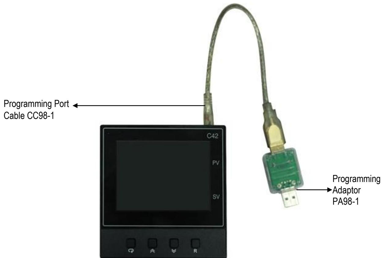
**1-4 Programming Port Connection with Programming Port Adaptor**
