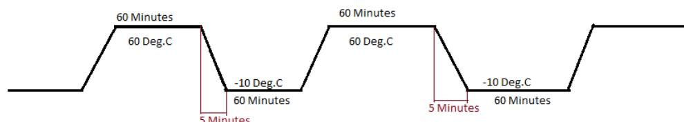
**4-5 Temperature Profile for Temperature Cycling Chamber**
