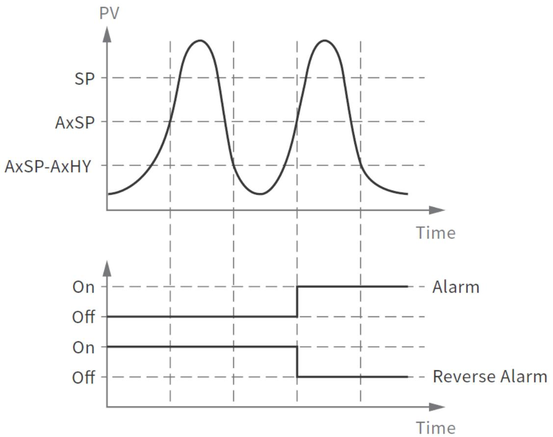
**3-20 Process Value High- Latching & Holding Alarm**
