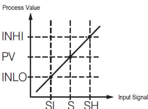
3-1 Conversion Curve for Linear Type Process Signal
