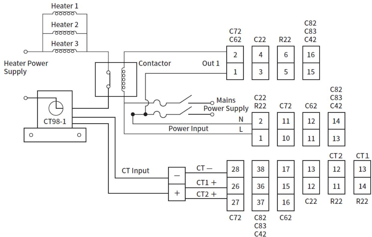
2-41 CT Input Wiring for Single Phase Heater
