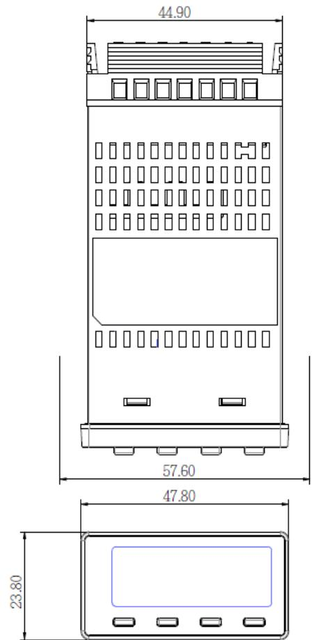
Recommended panel thickness is 1 to 5mm.
