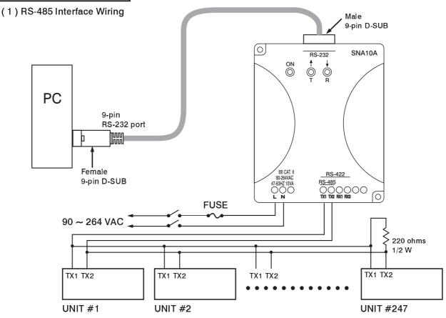
A 220 ohms 1/2 W termination resistor across the TX1 and TX2 terminals of the last unit in the network is required.
