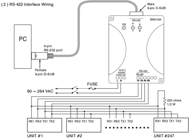
A 220 ohms 1/2 W termination resistor across the receive terminals of the last unit in the network is required.
