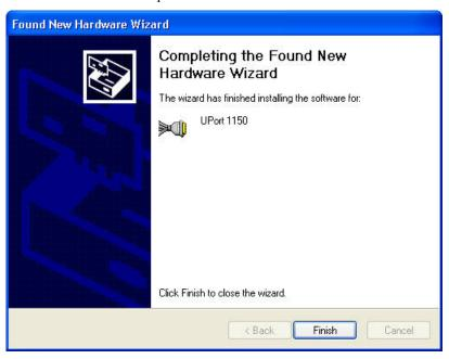
7. After Windows has completed installing the adaptor, it will automatically detect the new COM port. The **Found New Hardware** balloon will appear in the bottom right corner of the Windows desktop.
