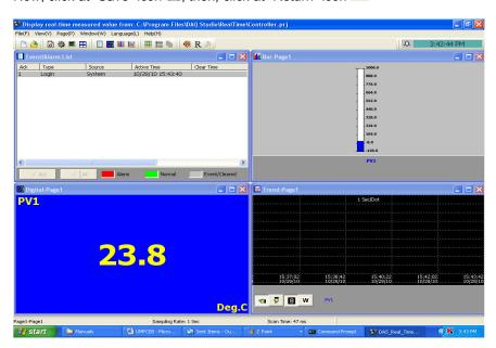
Check Scan time and sampling rate at bottom side of screen. Scan time is more than sampling rate, then, it generates communication error. If there are network delays or problems with communication settings, you may get communication error. In case if network delays, it is possible to modify sampling rate in DAQ software and then check again
