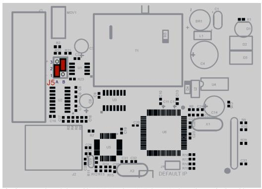
If J5 is setup as shown below, with J5A(2-3) and J5B(1-2) then a 120ohm active termination with  $\boldsymbol{Low}$  Line Idle will be connected to the RS485 network.
