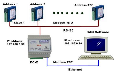
Note: Max. 127 IO modules can be connected in one RS485 network
