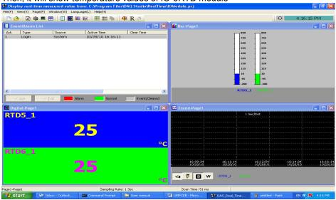
Check Scan time and sampling rate at bottom side of screen. Scan time is more than sampling rate, then, it generates communication error. If there are network delays or problems with communication settings, you may get communication error. In case if network delays, it is possible to modify sampling rate in DAQ software and then check again
