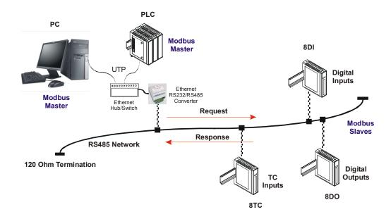
Fig: Max. 4 masters can access data of the IO modules via PC-E in Mode 0
