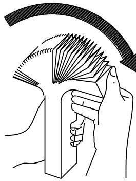
Fig. 5.5 Loosening the Chart Paper
