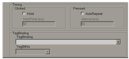
**Timing:** This is an advanced feature and used to make sure operator action is properly received by PLC when the PLC has a large scan time.
