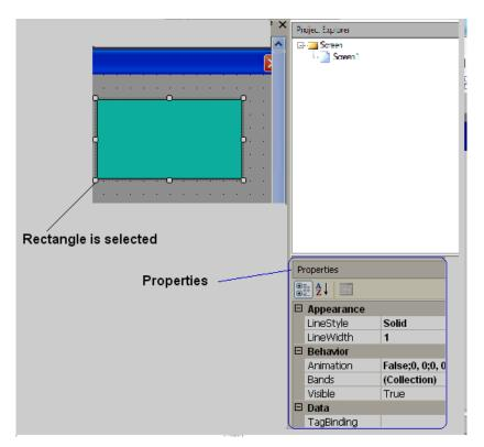
In above example, a rectangle is drawn, and once it is selected, the right side bottom corner will show all the properties for this specific rectangle if "properties" is checked in the View dropdown menu. It is possible to modify the properties of the rectangle from the property grid. Alternatively, if you double click on the rectangle, you will see a pop-up window where you can edit properties.
