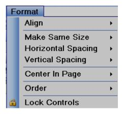
**1. Align:** Used to align selected components, objects etc. for adjusting their position precisely in the screen layout. Available options for selection are Center, Right, Left, Tops, middle & Bottom. Example: Align two Labels to the left in Recorder screen.
