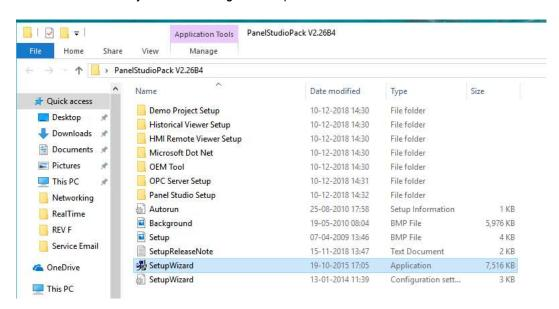
Select the required Software needs to be installed on the PC and press Install key to continue the installation.
