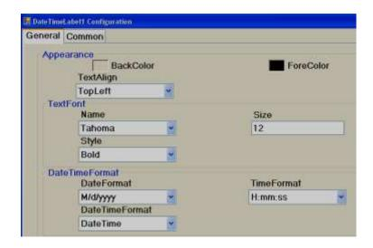
If date and time are required in more than one screen, it is better to create a screen and select the screen type as "Template", and then link this template to all other required screens to display Date and Time automatically. This is more efficient than keeping Date and Time label in more than one screen since it uses less memory.
