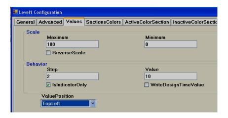
**Maximum:** This is the max range of the process value (analog input tag) **Minimum:** This is the minimum range of Process Value (analog input tag)
