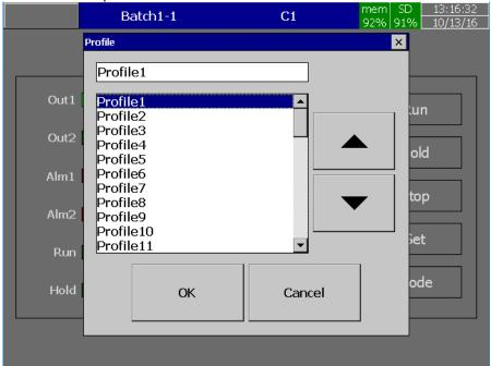
Press **Hold** to hold the profile. Press **Stop** to stop the Profile.
