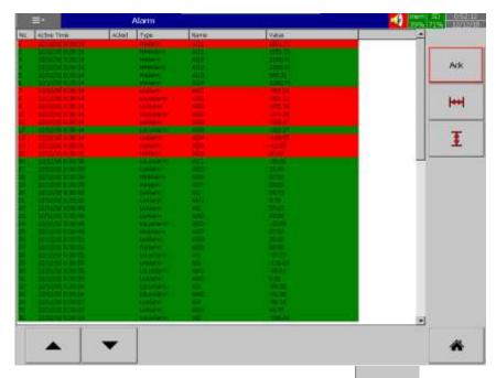
The user can acknowledge the alarm by pressing the ACK key. The user can navigate the alarm display by using the scroll keys . The user can go back to the Home screen by pressing the Home key. The user can access other menus by pressing the menu key.
