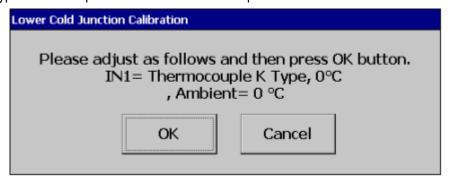
After input K type thermocouple with 0°C at ambient temperature 0°C, press ok, the user can see the below screen.
