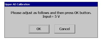
After input 5V, press ok, the user can see the below screen.
