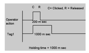
**Auto Repeat & Interval time:** This is generally applicable for a "Pressed" event. It is to repeat the action defined at the "Pressed" event as per the set interval time.
