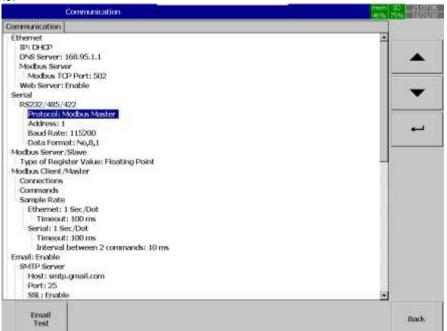
Configure the communication parameters as per the slave (controller) configuration.
