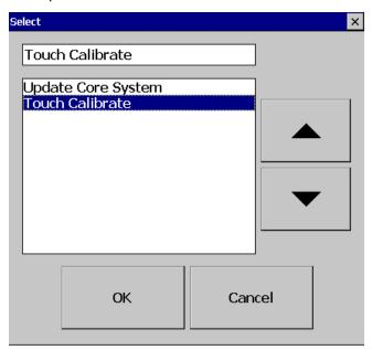
1. Select Touch Calibrate and press OK to do the screen calibration. The below screen will appear to do the screen calibration.
