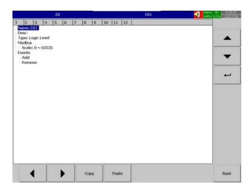
**Copy**: copy the channel configuration from one channel to another channel.
