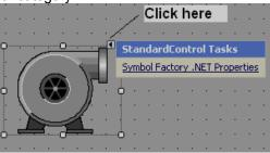
Drag and the drop symbol factory component onto a screen.
