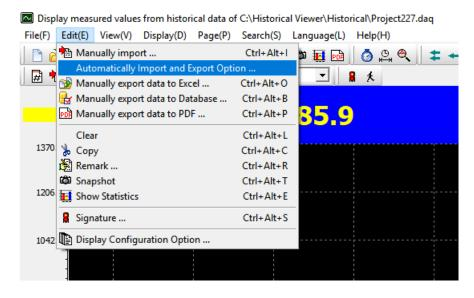
3. Select automatically, set the time interval, File path. The time interval can be set from 1 hour to 24 hours.
