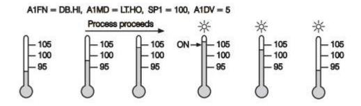
5-12 .Latching/Holding Deviation Band Alarm
