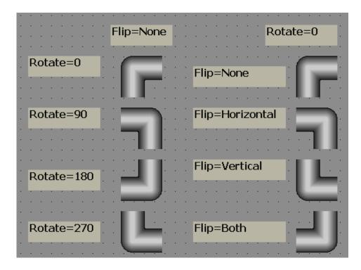
**Rotate**: Rotate symbol to any predefined direction in a specific band during Run time. Available options include 0°, 90°, 180° and 270°
