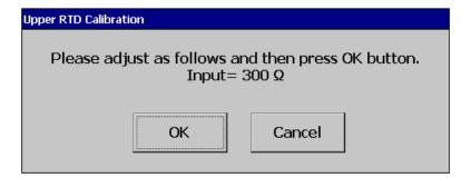
After input  $300\Omega$ , press ok, the user can see the below screen.
