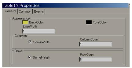
**Note:** Deselect "The same Width" to adjust column width in the Table **Note:** Deselect "Same Height" to adjust Row height in the Table
