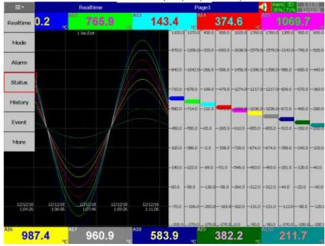
By using the DI, DO, AO, Counter, Totalizer tabs the individual status can be viewed in the respective tabs. The selected tab can be changed by using the left and right scroll keys.
