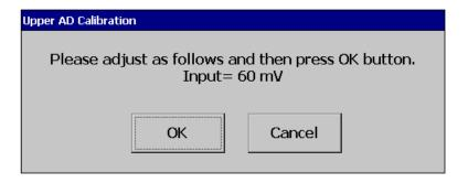
After input 60mV, press ok, the user can see the below screen.
