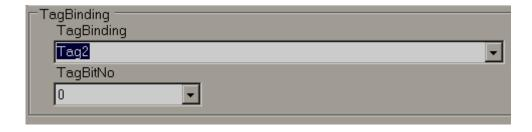
In the above figure, Tag2 is an analog type (4 bytes), so, a TagBitNo combo box will appear for the selection of the required bit within 32 bits (0 to 31).
