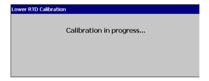
After successful calibration lower RTD calibration the system will request the user to input higher range input to the input channel.
