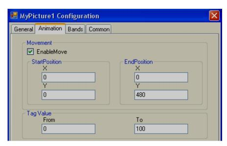
Ex: Recorder 7" (High Performance), Screen Resolution = 800 X 480, Horizontal installation, Width=800, Height=480. Move symbol from Left Top to Right Bottom on screen at an angle during Run time when the tag value changes from 0 to 100
