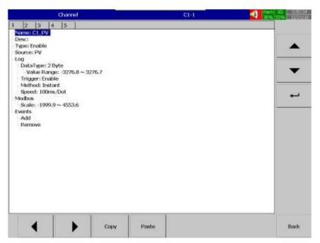
After entering the Configuration menu, in the Channel, select Controller then Press the Enter softkey to get into Controller Channel configuration menu. After entering particular controller configuration menu then selects channel then press Enter to enter into the controller channel configuration menu. It displays the Controller C1 channel C1-1(C1\_PV) as the first Controller channel configuration page. Press directional navigation keys
