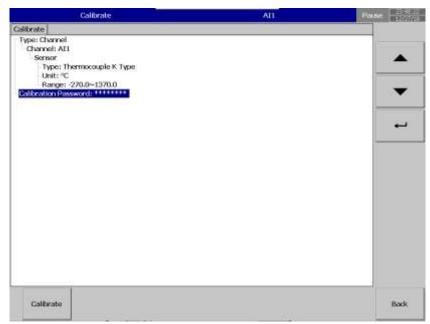
**Type:** Choose Channel for calibrating Analog Input and Analog Output, Controller for calibrating PID process control card input.
