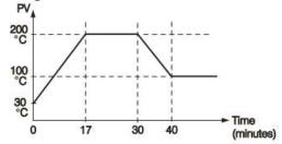
**Note**: When the ramp function is used, the lower display will show the current ramping value. However, it will revert to show the setpoint value as soon as the up or down key is touched for adjustment. The ramping
