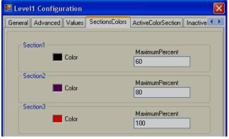
**Sections colors:** It is configured bands for the sections to show different colours for Labels and Ticks in the Level graph.
