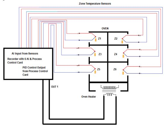
To achieve this function set the following parameters in the PID Control setup menu and configure the Recorder as per the recording requirements.
