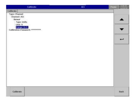
The system will prompt for a user conformation to do the calibration of the channel.
