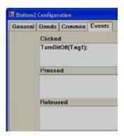
When the operator clicks Button1, Tag1 will = 1. Now, Tag1 will = 1 even after the operator releases the button, and it will continue to maintain its earlier state. When the operator clicks Button2, Tag1 will = 0.
