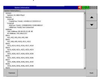
The System Information page contains softkey to access Touch Screen Calibration and Firmware upgrade Menu.
