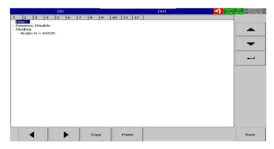
**Copy**: copy the channel configuration from one channel to another channel.
