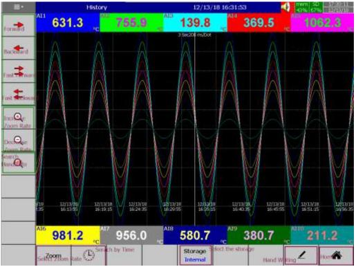
The historical display page will allow the user to navigate the historical data and do the handwritten remarks on the display page. The user can do the navigation on the screen using the four scroll keys. The user can increase or decrease the zoom rate by using the two softkeys. The handwritten messages within the data can be searched by using key. The zoom rate can be selected by using the softkey.
