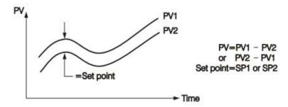
The PV display will indicate PV1-PV2 value if P1-2 is chosen for PVMD or PV2-PV1 value if P2-1 is chosen for PVMD. If the user needs PV1 or PV2 to be displayed instead of PV, they can use the Display Mode to select PV1 or PV2 to be viewed. If PVMD selects P1-2 or P2-1, while SPMD selects PV1 or PV2, an Error Code will appear. In this case, the signals used for input 1 and input 2 should be the same unit and same decimal point, that is, IN1U=IN2U, DP1=DP2, otherwise, Error Code will appear.
