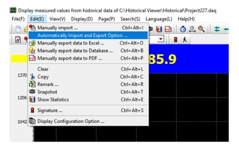
2. Select automatically and export to excel or automatically and export to database format or automatically and export to PDF, set the time interval, File path and File attributes. The time interval can be set from 1 hour to 24 hours. The file attribute can be written to single file or multitude files.
