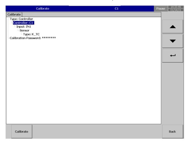
Type: Choose Channel for calibrating Analog Input and Analog Output, Controller for calibrating PID
