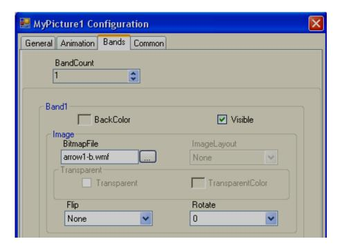
**Band Count**: Used to define bands for run-time animation of the symbol. Max. 32 bands are supported.
