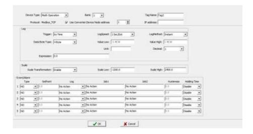
5. Linear Channels for 3<sup>rd</sup> party Modbus slave devices to connect via Modbus protocol.
