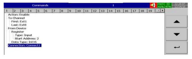
5-21 Mapping of IO Module and External Channel for Slave ID2
