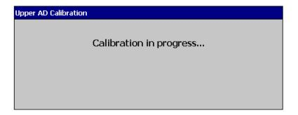
After successful calibration of upper AD calibration, the system will prompt the user to connect the input as K type thermocouple with 0°C at ambient temperature 0°C.
