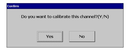
Press Yes to do the Calibration on No to exit. The system will inform the user to input the low-value input to the channel.
