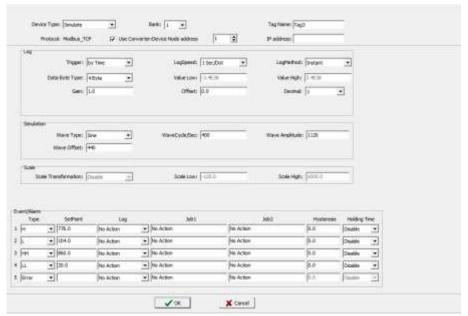
All the channel configurations are similar to recorder channel configuration. Every channel can be configured with 5 different types of events or alarms similar to the recorder and each event can be configured with two jobs.
