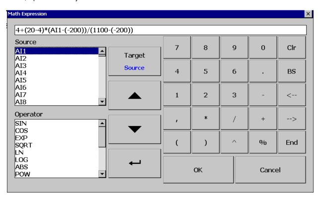
The Source consists of all available Analog inputs, Digital Inputs, Math inputs, external channels. The Operator consists of available mathematical expressions. Use Source, Operator and keyboard to define the Math equation.
