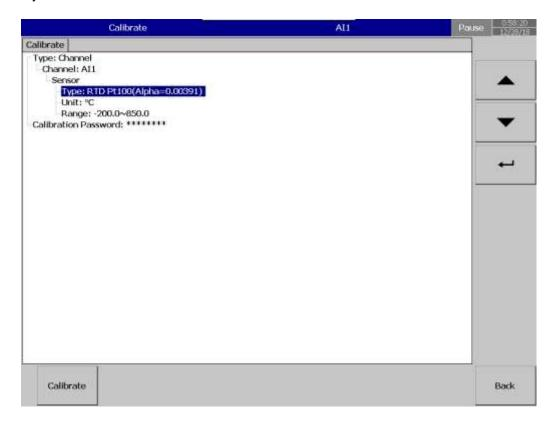
The system will prompt for a user conformation to do the calibration of the channel.
