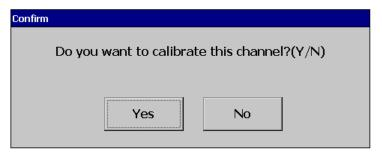
Press Yes to do the Calibration on No to exit. The system will inform the user to input the low-value input to the channel.
