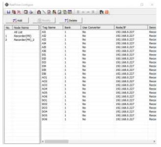
8. Close the Real-time configuration viewer to update the tag contents and logging the data from the configured devices to PC. The configuration Viewer can be closed by pressing the X key on the right side top or key.
