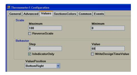
**Maximum:** This is the maximum range of the Setpoint (Analog Tag, Normally this is an Analog input, 20 mA, 10V DC etc.)
