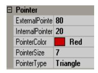
**External Pointer Radius:** It is used to set an external pointer Radius, define end position. **Internal pointer Radius:** It is used to set the Internal Pointer Radius, defines start position.
