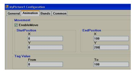
Movement: Select the Enable/Move checkbox, then, enter the X and Y start and end positions
