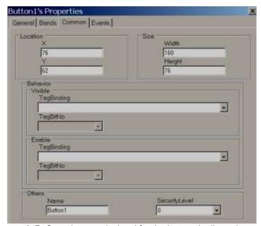
**Security control:** Defines the security level for the button. It allows the user to operate the button only when the operator security level is equal to or more than the security level defined here. Please refer section "Security" at Project explorer for more information about security features.
