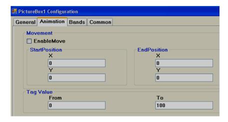
**Movement:** Select "Enable Move" if it is required to move picture during Run time from Location 1 to Location 2 based on a tag Value. Start and End coordinates for X and Y needs to be configured during Design time, and the Picture moves in Run time based on a Tag value.
