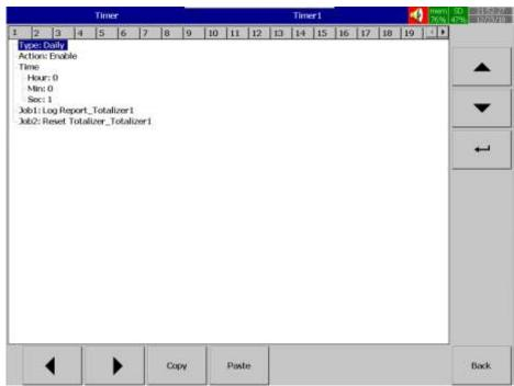
The timers can be used to execute a job on a time basis. The timers can be categorized into Countdown, Repeat Countdown, Daily, Weekly and Monthly.
