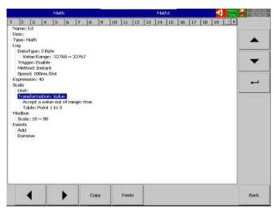
The scale low and scale hi of the math channel can be referenced from transformation table output values. For example, the transformation table configured as below.
