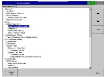
Configure the communication parameters as per the slave (IO Module) configuration.
