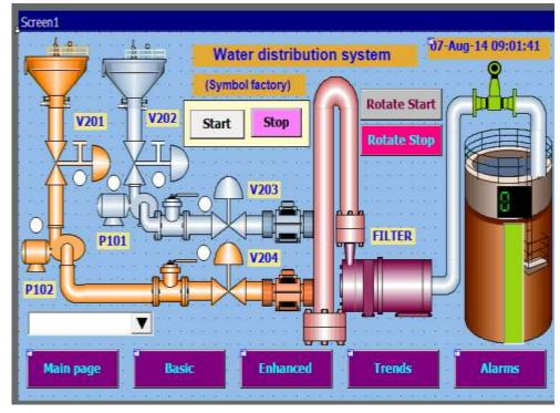
Use this editing software to develop custom screens on the Recorder. It is mainly used for application development for operator interface in industrial applications such as display real-time value of process parameters like temperature, flow, pressure, visualize process data in meaningful ways such as bar graphs, dial, meter, level, digital LED, animation like visibility control, blinking, horizontal movement, vertical movement etc.
