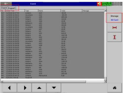
The Event power can be navigated by using the scroll keys . The stored location of displayed historical events can be switched between internal memory and SD card by using the softkey .
