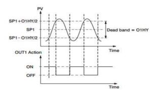
The ON-OFF control may introduce excessive process oscillation even if Hysteresis is minimized to the smallest. If ON-OFF control is set (i.e. PB1 = 0), TI1, TD1, CYC1, OFST, CPB and PL1 will be hidden and have no function to the system. The manual mode, auto-tuning, self-tuning and Bumpless transfer will be disabled too.
