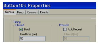
If a button is not switching properly at the PLC, then, in the "General" tab, select the "Hold" checkbox and enter the hold time. The default value is 50 msec. If required, adjust this to 100 msec. and check again if the button is switching properly.
