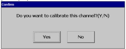
Press Yes to do the Calibration on No to exit. The system will inform the user to input the low-value input to the channel of the process control card.
