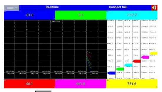
❖ By using the menu key various real-time pages, the status of DI, DO, AO, Counter and Totalizer, the real-time alarm on the recorder can be viewed.
