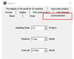
**Sampling rate:** It is used to set data display time for Real-Time Viewer. User can select One from the following for real-time monitoring.
