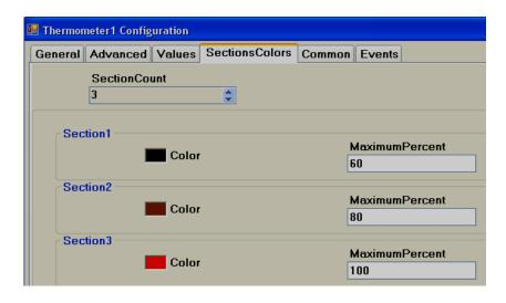
**Section Colors:** Define bands to display Ticks and Label colour accordingly based on the value of the tag during Run time.
