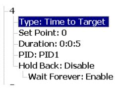
This is similar to the ramp segment with automatic calculation of ramp rate by the Process Control Card with the reference of Setpoint and duration given by the user.
