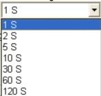
**Time out:** This is time set for generating time out errors related to real-time viewer Communication.
