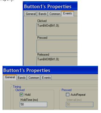
If the button is not switching properly at PLC, then, in General, Tab, select "Hold" checkbox and enter the hold time. The default value is 50 msec. If required, adjust this to 100 msec. and check again.
