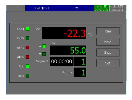
The real-time display page will show the Profile and Segment no along with the remaining time of that particular segment.
