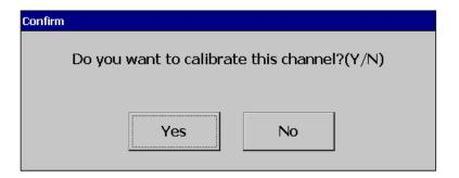
Press Yes to do the Calibration on No to exit. Connect a Current measuring meter before starting calibration.
