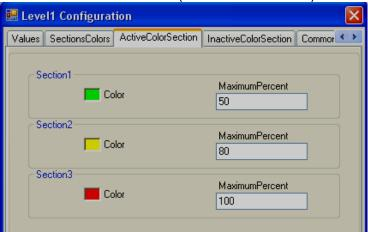
**Active Color Section:** Defines the active colour for the process value band. For example: If a process value range is 0-100, set different bands in % for the process value, and define colours to appear within the level Bar graph during Run Time.
