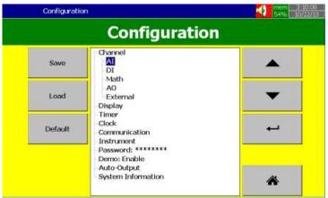
Press (Menu), then More and then Config softkey to enter Configuration mode. In the Configuration screen, select "Communication", then press the "Enter" softkey.
