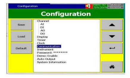
After completing the above steps, press the "Back" key, then the "Home" key to return to the main menu. It will save the configuration settings in the Recorder. Now the Recorder is ready for the Web Server Applications.
