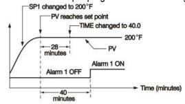
**Note:** The TIMR can't be chosen for both A1FN and A2FN simultaneously; otherwise an error code will produce.
