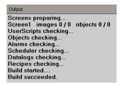
After creating a build, if any errors are shown at Output window, do not attempt to download the application from PC to Recorder, or PC to USB flash disk first clear the errors and make sure that compilation errors are not present before transferring the application to the Recorder.
