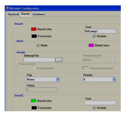
Bitmap file: Select the image to be displayed when the tag value reaches this band in run time.
