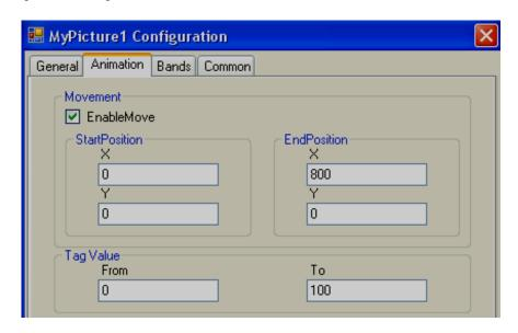
To move the symbol from Left to Right, set start and end Positions for X coordinate in pixels, there is no need to set Y coordinates.
