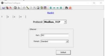
5.2. If the device is connected to PC via RS232 or RS485 port then configure the bank with Protocol as Modbus\_RS232 and other communication parameters such as comport no, Baud Rate, Parity, Data Bits and Stop Bits as per the connection.
