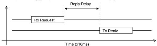
Note: From Version 8 onwards, reply delay works only when dipswitch10 is ON that means when user defined communication settings are used.
