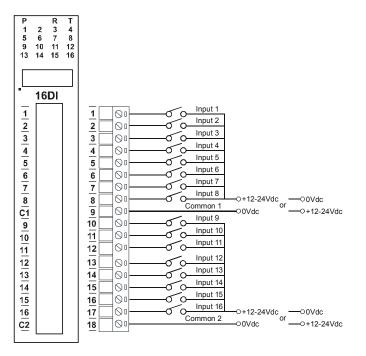
The following diagram shows how the digital inputs are connected a NPN transistor or a PNP transistor.
