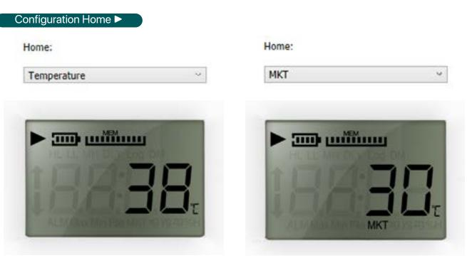
Users can set home page to display temperature, humidity, max/min temperature, or MKT.
